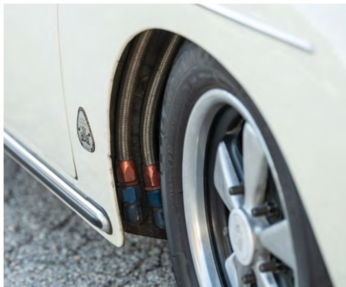
Fuchs wheels and braided oil cooler lines were not standard equipment on a 1959 Convertible D.
