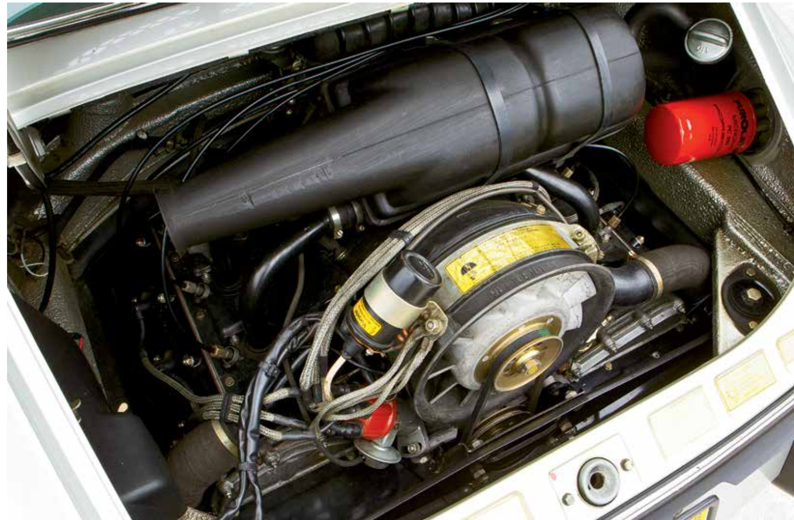
Above: The 2.4-liter flat six, with its newly developed Bosch CIS fuel injection, produced 140 horsepower and gave the 911 a top speed of 130 mph.
